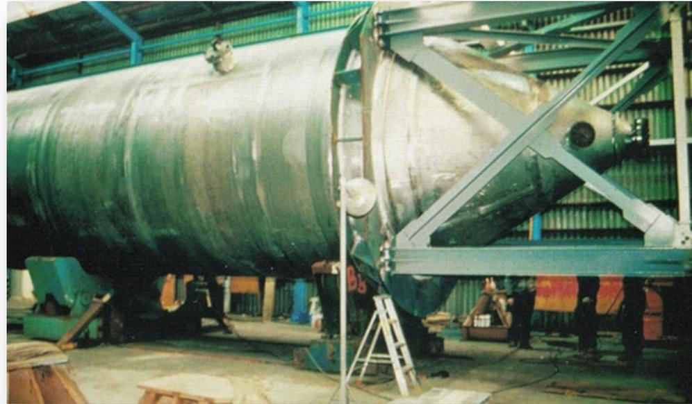
**Cellulose digester built in duplex stainless steel 1.4462 (2205)**
