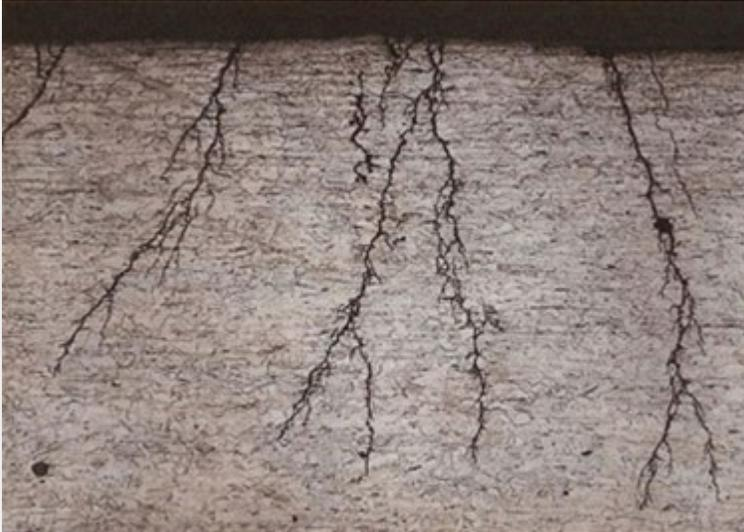
**Cracks, typically branched, have extended for 4 mm, plate thickness 5 mm**
