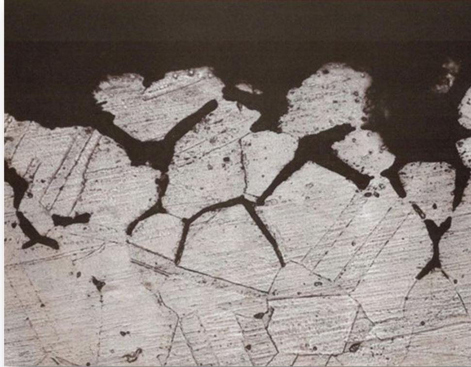
**Intergranular corrosion in a pressure vessel after faulty heat treatment which causes precipitation of chromium carbides**
